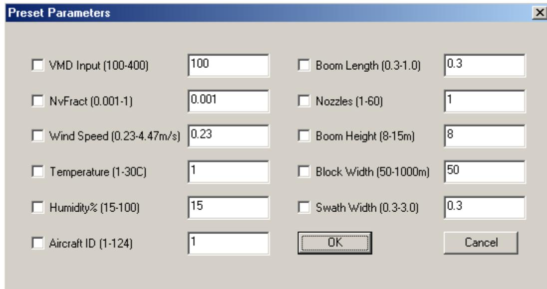
Figure 2. The Interface to Preset Spray Parameters
