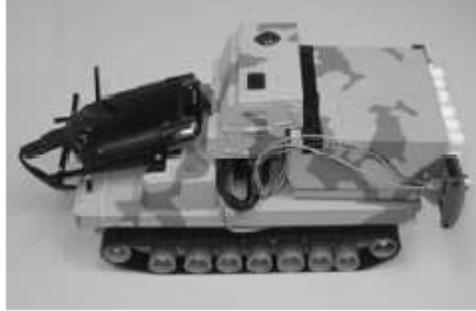
Figure 3.6 The Modified Tank Chassis
