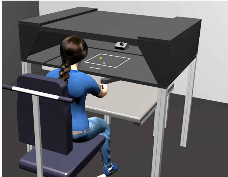
Figure 3.1: A research participant seated at the KINARM End-Point Lab with a monocular EyeLink 1000 eye tracker. Reprinted from Barany et al., 2020.
