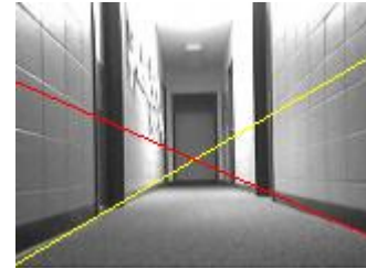
The final result of applying the Hough transform after the feature extraction process.
