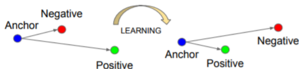
Figure 3.1: Diagram of the relative distances between triplet points. The distance between the anchor and the positive point should be minimized and the distance between the anchor and the negative point should be maximized. (Source: Schroff et al., 2015)
