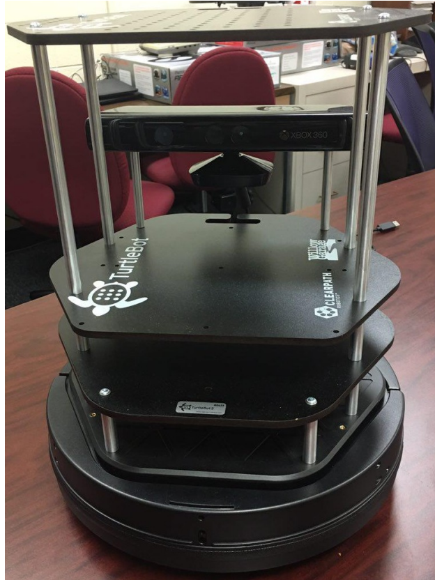
Figure 5.7: This is the Turtlebot that has been used on our experiment. Each Turtlebot is equipped with a Microsoft Xbox 360 Kinect, which provides a camera, a ranging sensor, and a microphone.
