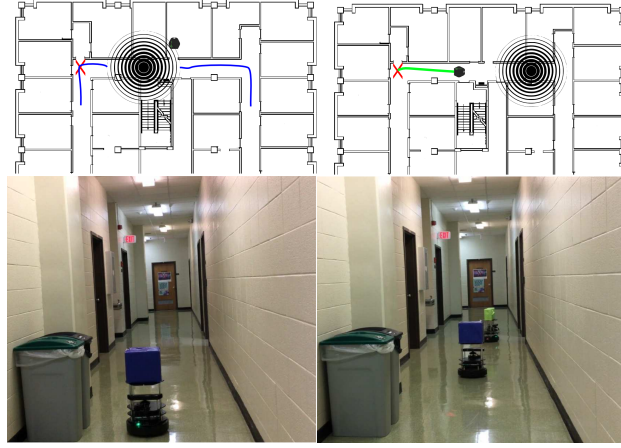
Figure 1.1: The top two images are our experiment in the simulation. We used ROS to run the simulation. The patroller securing the hallway and concentric circles around the patroller is an indication of the magnitude of the sound intensity. As the distance between the patroller and the intruder increases the intensity decreases. The lower images are from the physical experiment done with two Turtlebots. The two images on the right-hand side shows the moment that the intruder attacks and the two images on the left-hand side show the observation time.
