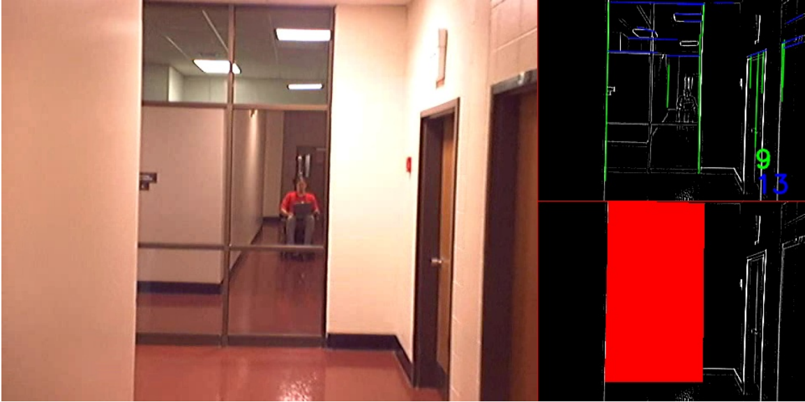
Figure 5.4: False Positive – rectangular region detected as doorway candidate
