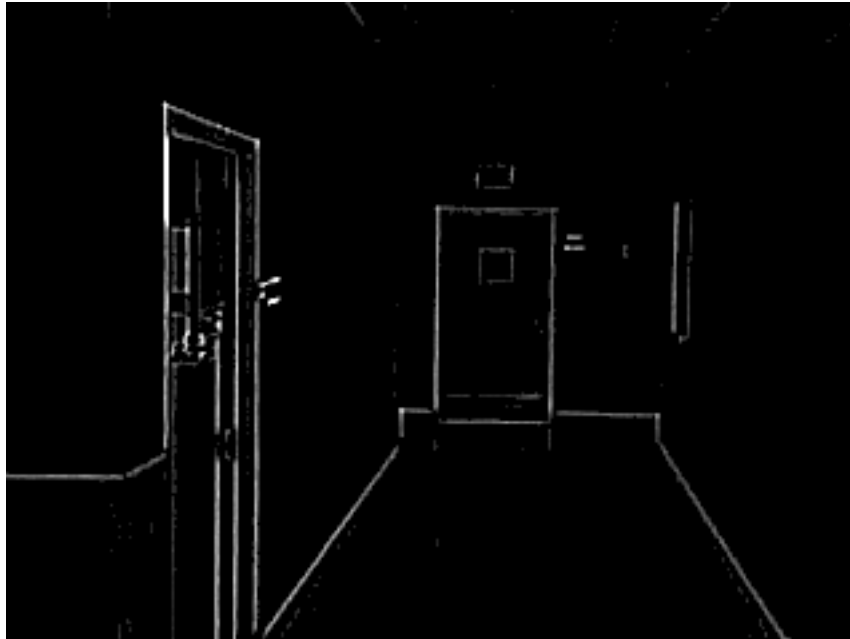
Figure 4.3: Results of Laplacian Edge Detector
