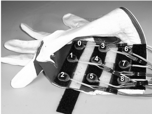
(a) The layout of the vibrotactor array on the back side of the glove.
